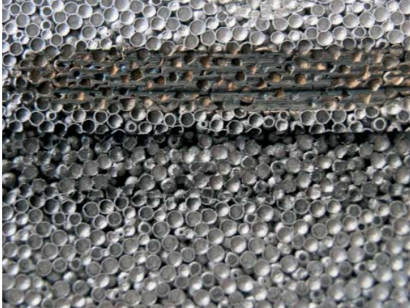
Fig. 3: Detailed hollow-sphere structure after the abrasion test.
