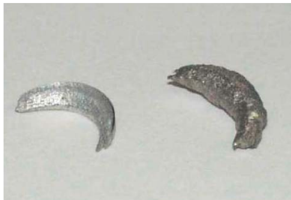
Fig. 2: Nibbled and punched granulate particles, before and after foaming.
