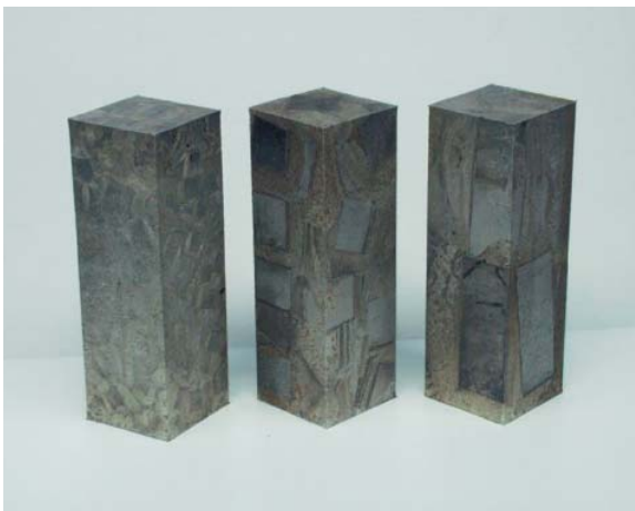
Fig. 4: Examples of different granulates and the foam objects made from them.
