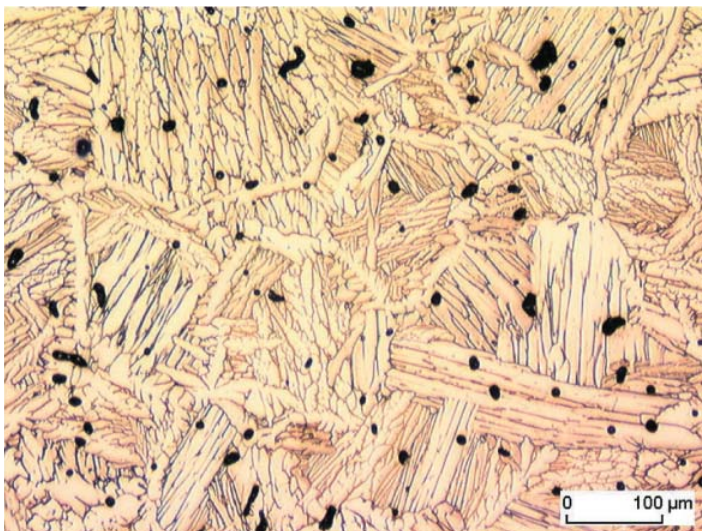
Fig. 1: Micrograph of a sintered TiAl6V4 sample made from a powder mixture.
