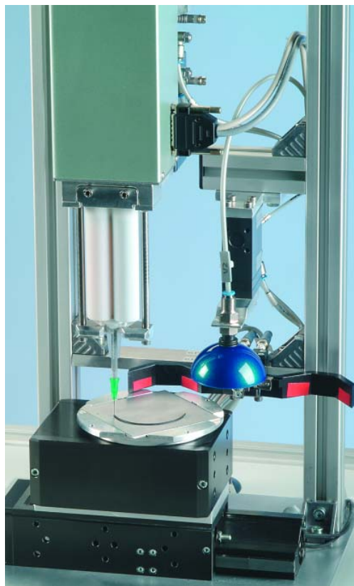
Fig. 3: Precision dosing unit for automatic application of 2-component adhesives from twin cartridges (IFAM development).
