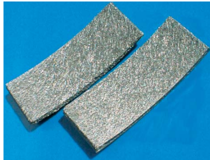
Fig. 1: Test sample of sintered Aluchrom YHf fibres.
