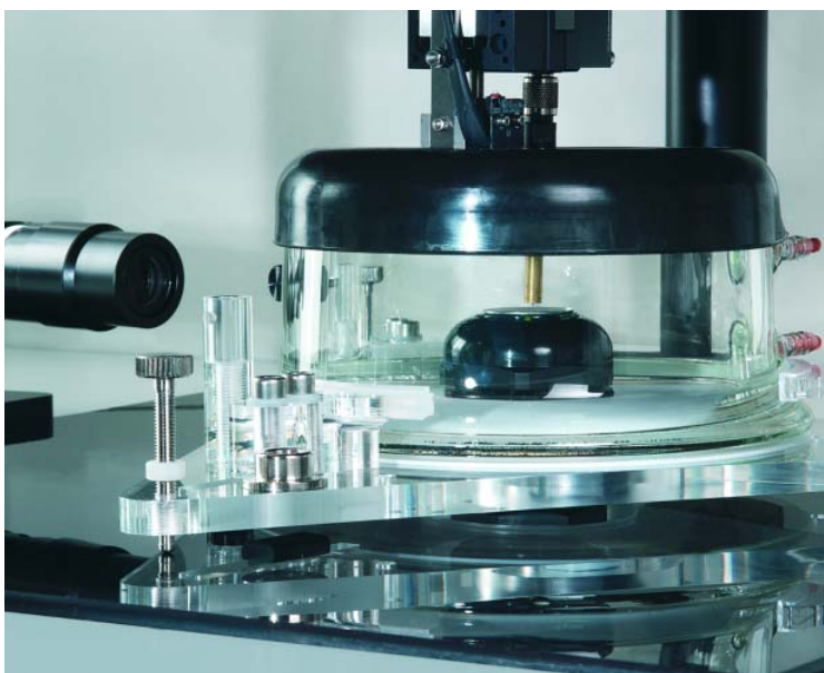
Fig. 3: Close-up of the scanning Kelvin probe.
