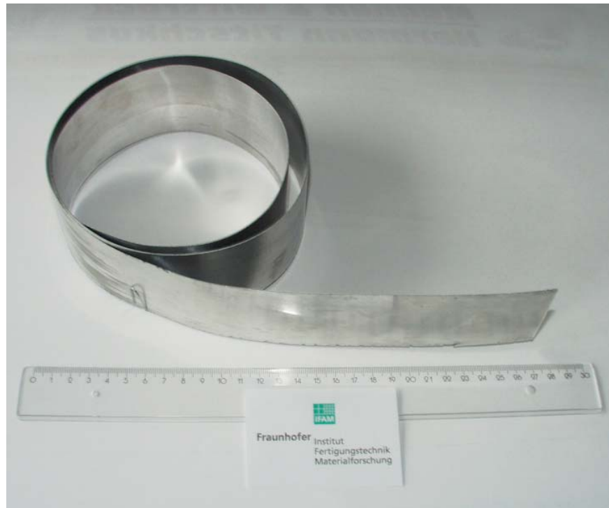
Fig. 1: Foamable aluminium semi-finished product (coil) manufactured by cold-isostatic pressing, sintering and rolling.
