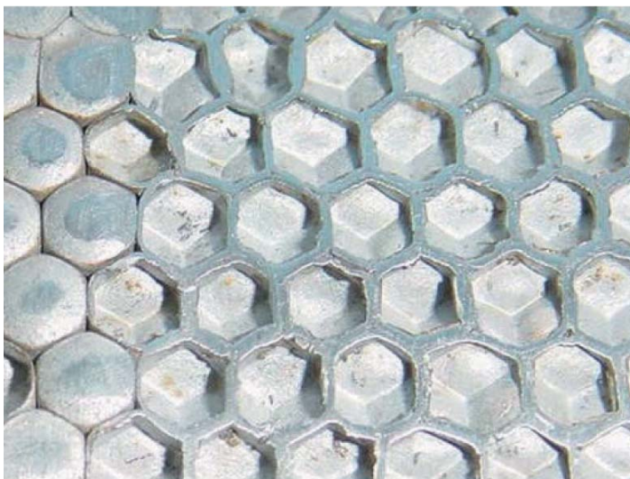
Fig. 3: Regular cellular metal structure manufactured via hollow sphere technology.
