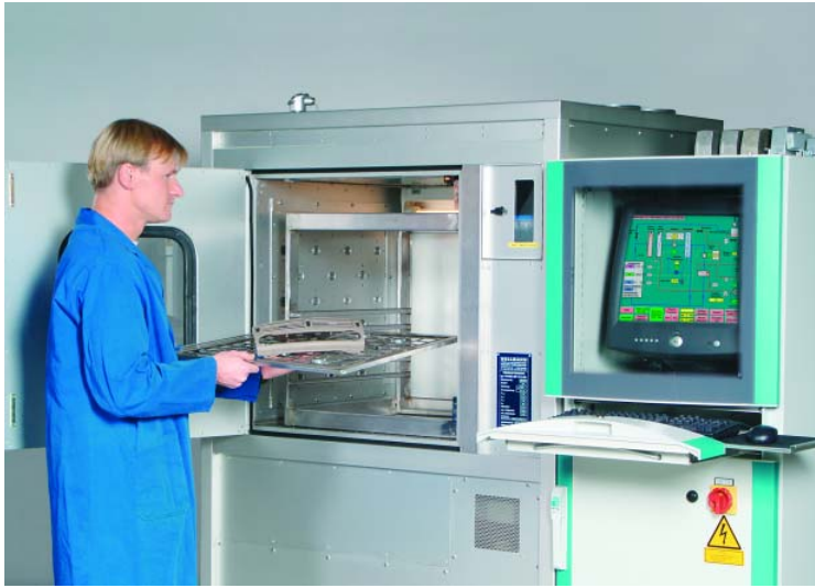
Fig. 1: Unit for drying paint/lacquer with moisture-free air (cold dryer).
