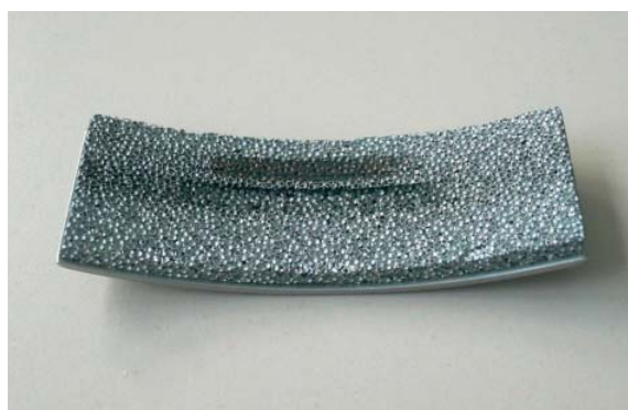
Fig. 2: Hollow-sphere structure after the abrasion test.
