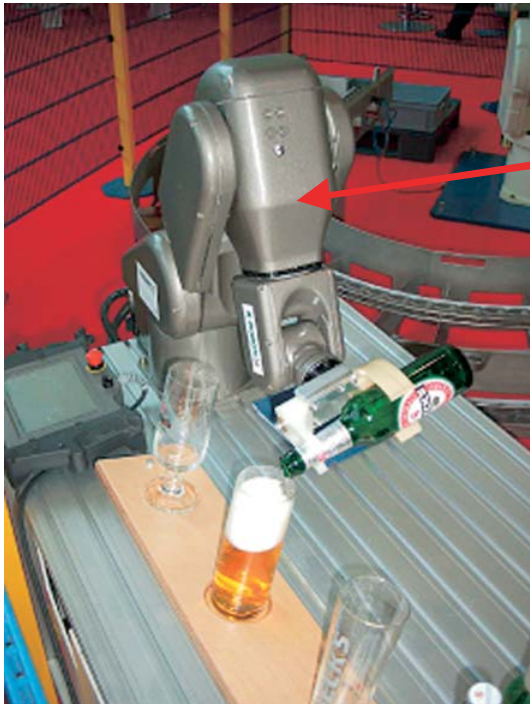
Fig. 1: A robot used in the food industry (left) is coated with a paint having an Ag-filler. The anti-bacterial effectiveness could be proven using a biotechnological test method (right).
