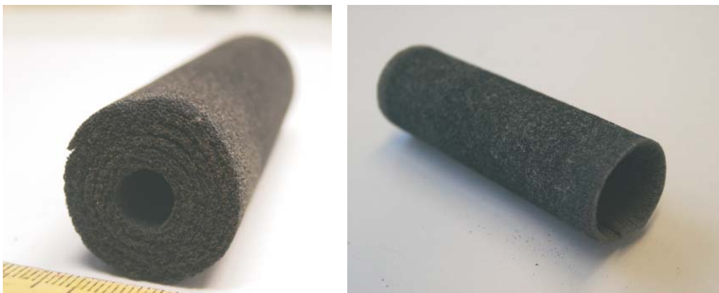
Fig. 3: Worked foam structures made of NiAl.
