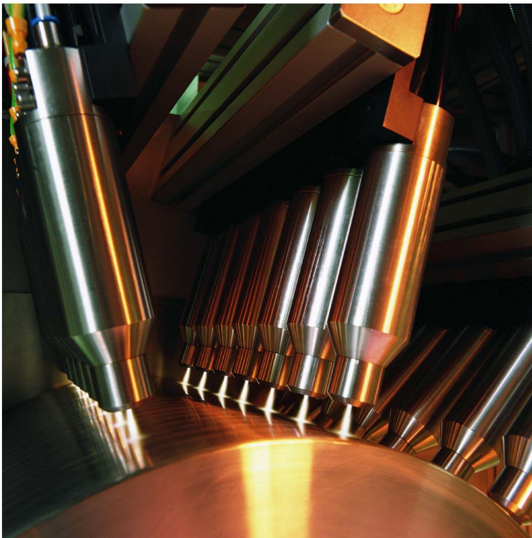
Fig. 4: Atmospheric pressure plasma unit. The nozzle assemblies are configured for simultaneous activation of several separate treatment tracks.
