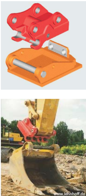
Fig. 1: Demonstrator object: "Quick-changer" (left: principle, right: in actual use).
