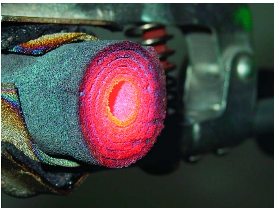
Fig. 5: Test on a NiAl structure at 1,050 °C (air).
