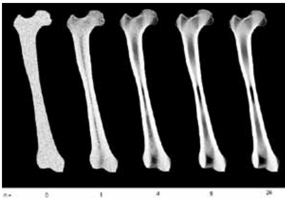
Fig. 3: 2-D simulation of the “Bone Remodelling” procedure in a human femur while the person is standing on one leg. After 24 iterations, we obtain a bone density distribution in close compliance with an X-ray image of a real bone.
