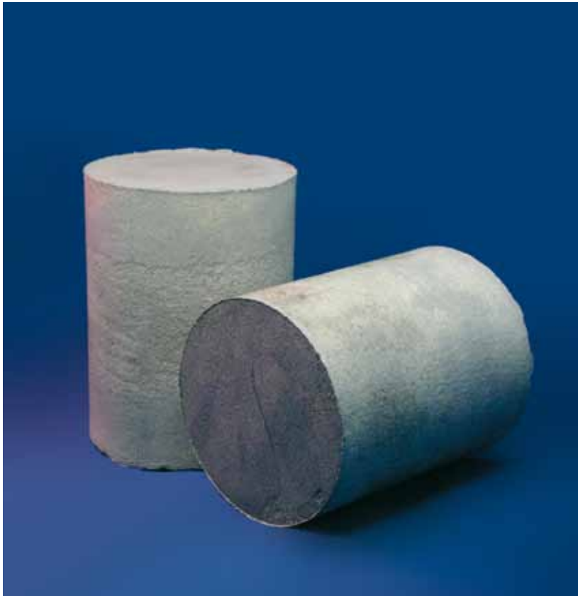
Fig. 2: Bolts compacted by means of Spark Plasma Sintering (SPS), made of an atomised aluminum alloy ( \varnothing 75 mm, height 85 mm, almost 100 % of calculated density).
