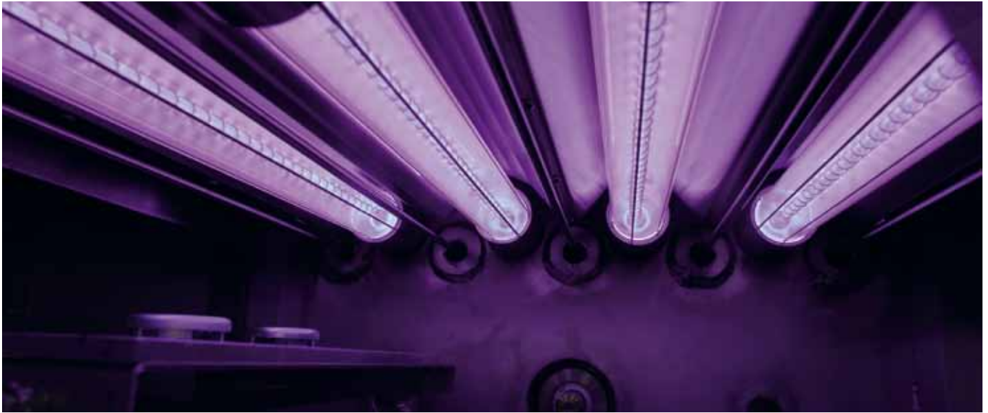
Fig. 5: Internal view of the VUV excimer plant.
