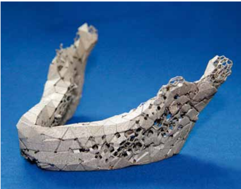
Fig. 5: Human lower jaw with biomimetically graduated cellular structure, made by SLM (metallic bone foam).
