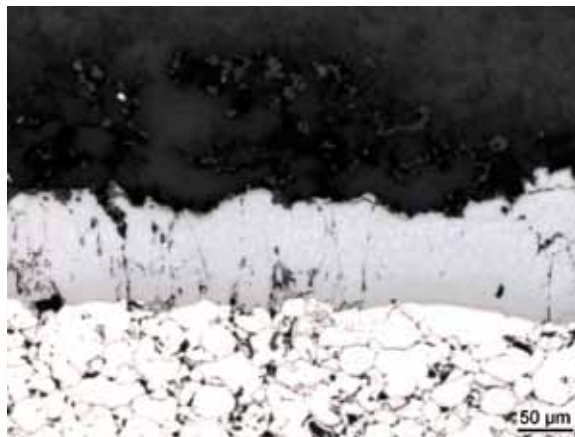
Fig. 1d: Powder metallurgical pressed steel 316L, coated with copper-alloyed aluminum-powder.
