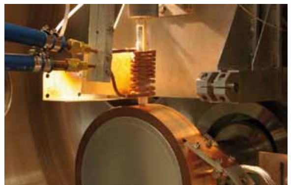
Fig. 1: Melt spinner to produce metallic materials of homogeneous characteristics.
