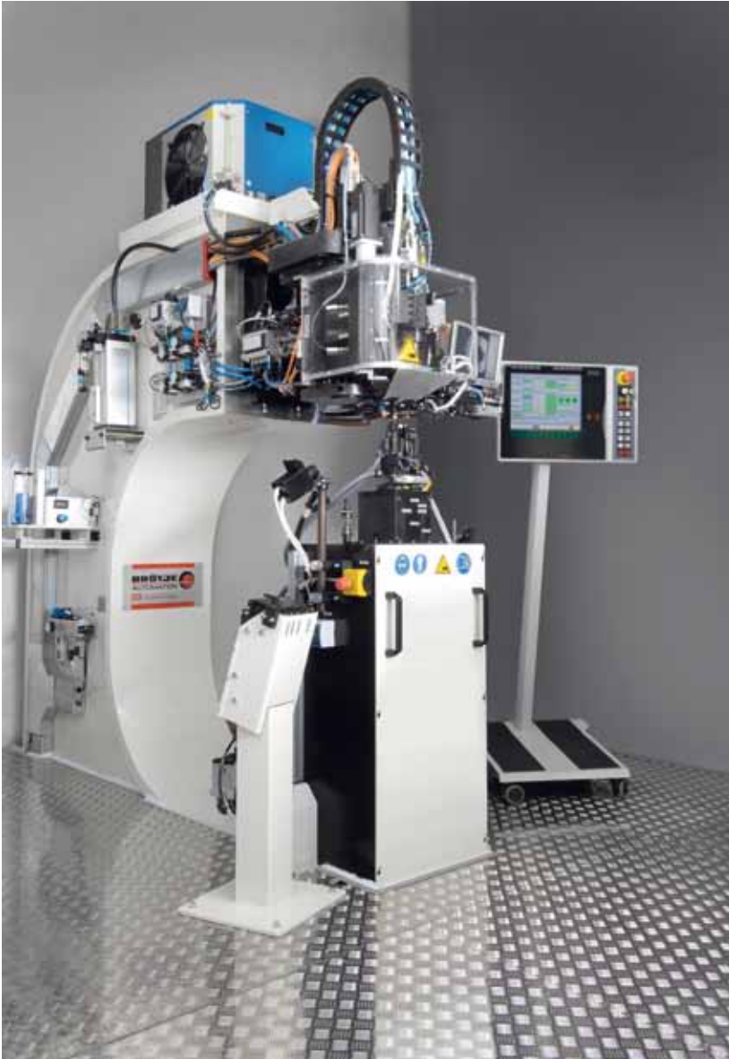
Fig. 2: C-frame automatic riveting machine of the Fraunhofer IFAM.
