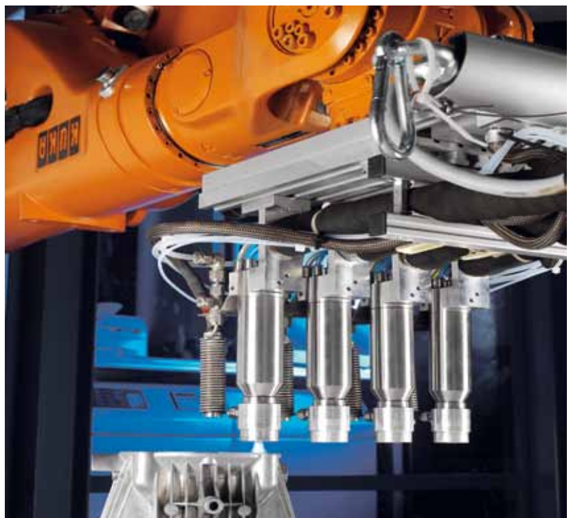
Fig. 3: Corrosion protection for aluminum pressure-die casting components using atmospheric pressure plasma technology (AP plasma technology).
