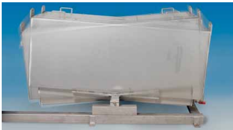
IMO test chamber for measuring corrosion for applications on ballast water tanks.
