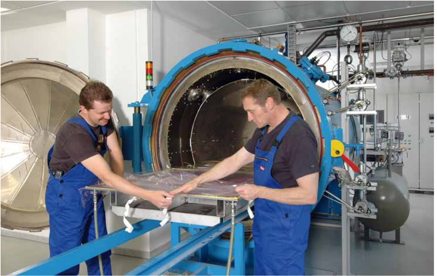
Fig. 3: Autoclave for manufacturing fiber reinforced plastics.
