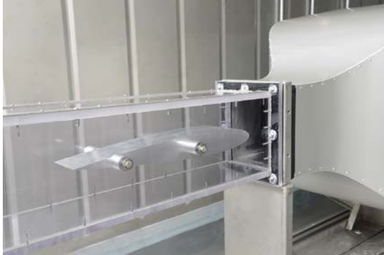
Test zone with integrated wing section.
