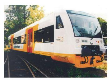
When joining by adhesive bonding, GFRP material properties (high stiffness with comparatively low weight) are retained! The adhesive bonding process has made it possible to make optimum use of the GFRP lightweight construction properties and to build the "RegioShuttle" 25% lighter than comparable conventional steel vehicles.
