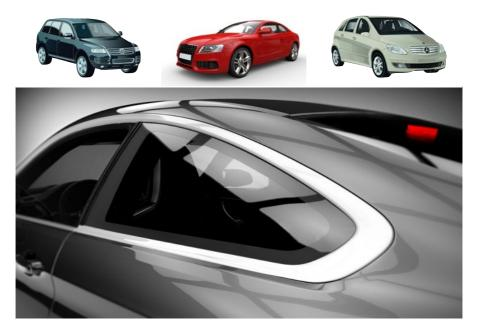
entire bodywork. The advantage is that the adhesively bonded joint between the windscreen and the bodywork increases the torsional stiffness of the vehicle by 15-20 % compared to the inserted window. This, in turn, makes it possible to use thinner, i. e. lighter, sheets of metal and results in a weight reduction of the vehicle.
