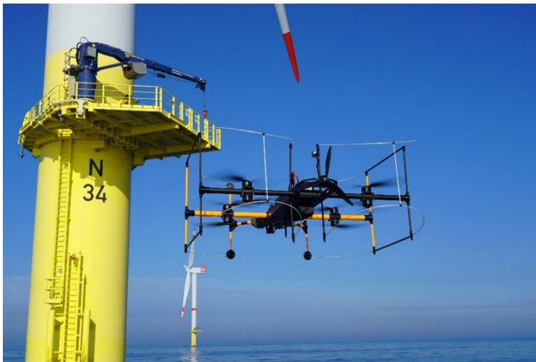
UAS deployment for the inspection of an offshore wind turbine as part of the research project AIDA. Supported by the Federal Ministry for Economic Affairs and Climate Action on the basis of a decision by the German Bundestag, Grant: 03EE3057A. © Fraunhofer IFAM
