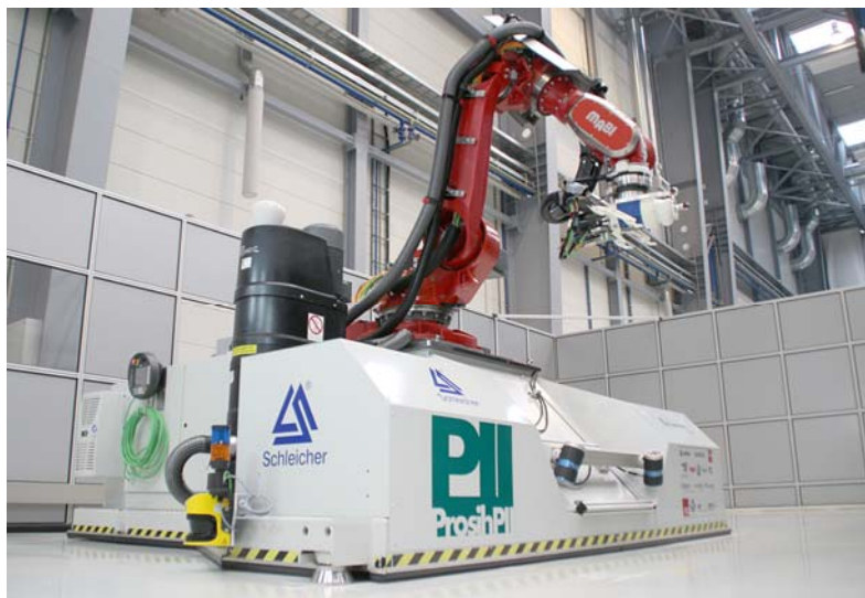
Mobile CNC robot for machining large structures. © Fraunhofer IFAM
