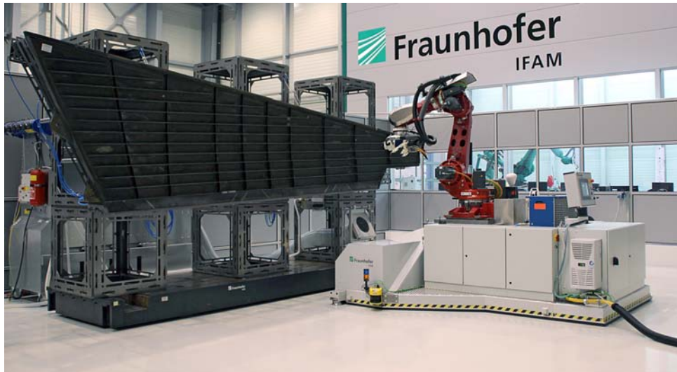
ProsihP II system machining a shell of an A320 vertical tail plane. © Fraunhofer IFAM
