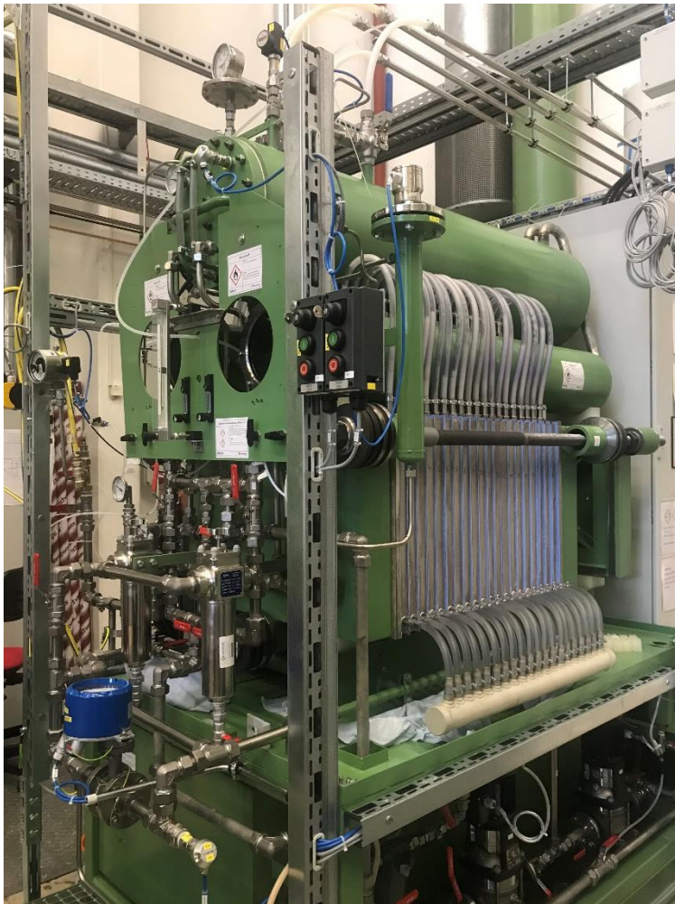
Picture 2: Industrial alkaline atmospheric test electrolyzer at Fraunhofer IFAM Dresden
