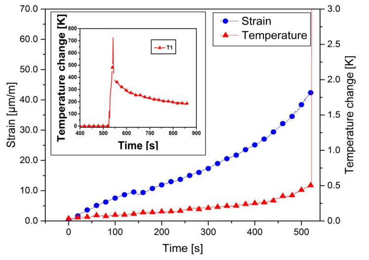
increases fast, while the temperature has a low increase, until the thermal runaway takes place.
