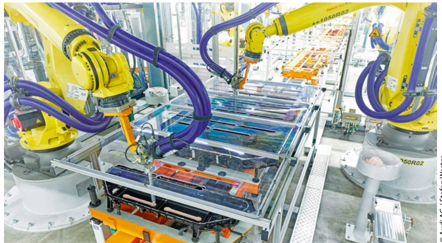
Figure 1 > Before inserting the cell modules into the compartment floor, a heat-conducting gap filler is inserted.
