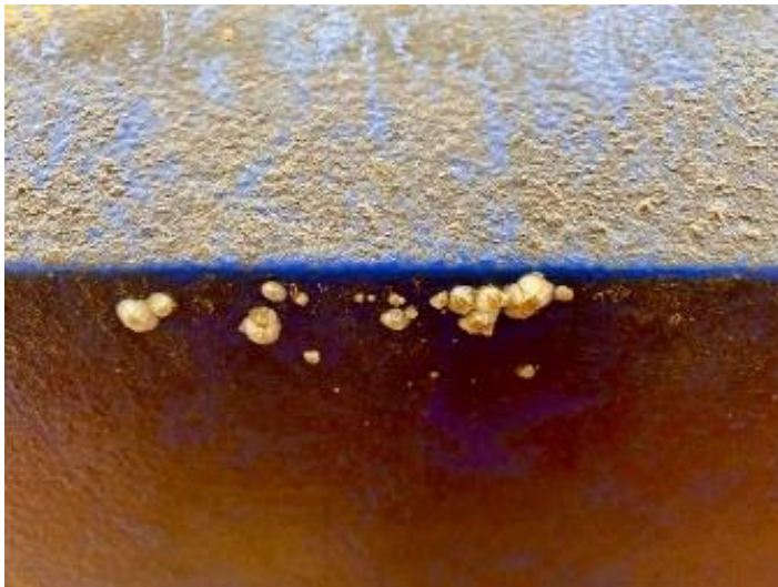
Ship's hull in the dock: Barnacles and dried biofilm – typical traces of maritime fouling. © Fraunhofer IFAM
