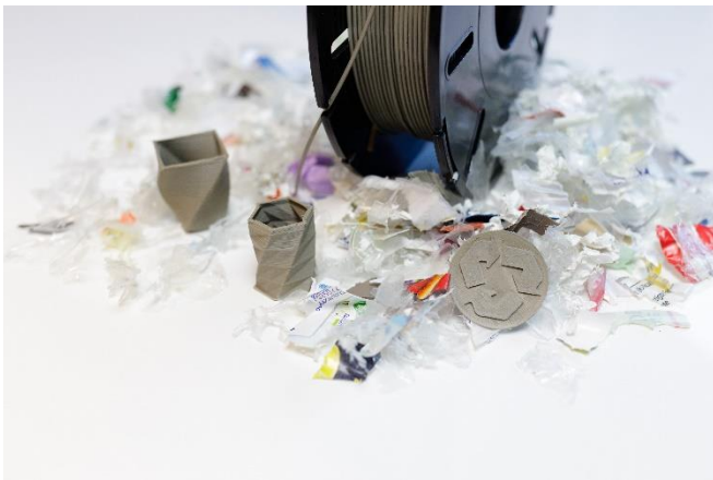
Fig. 2 Prepared material for additive manufacturing: Post-consumer waste is processed into filaments for 3D printing.
