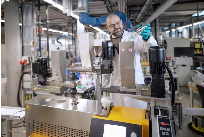
Fig. 1 The cleaned plastic packaging waste is mixed, melted down and extruded in a compounder at Fraunhofer IFAM.
