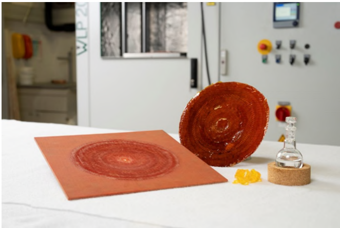
Fig. 1 The moldable, recyclable polymer patch can take on any desired shape and size.
